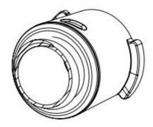
Twist 90 degrees clockwise to lock in place.
